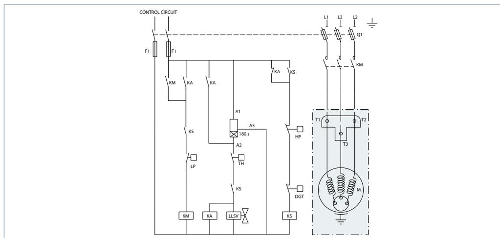
**Wiring diagram without pump-down cycle**
