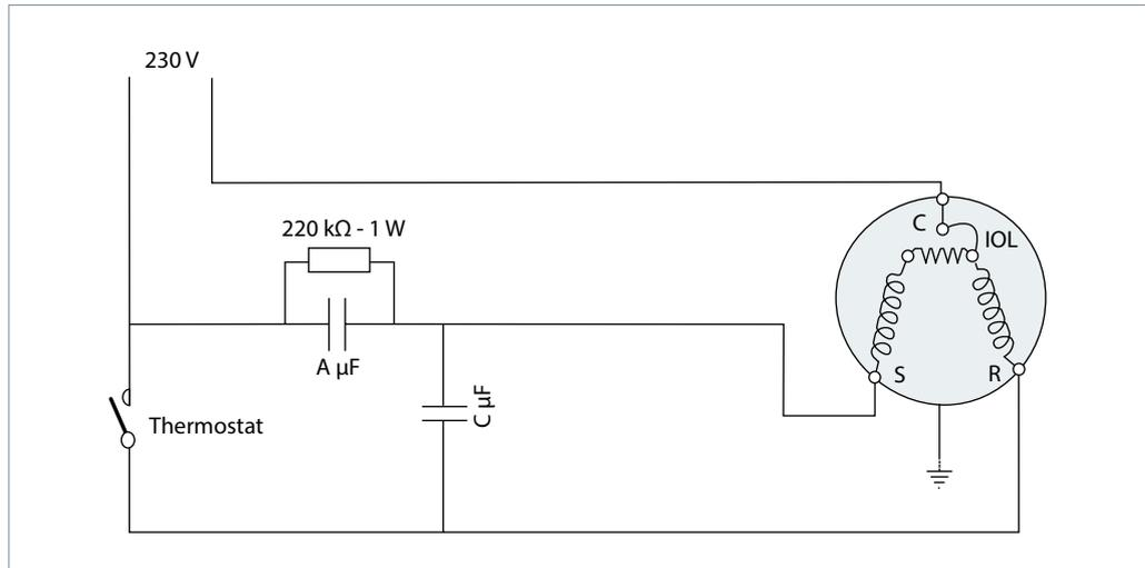
**Single phase - CSR wiring with trickle circuit**
