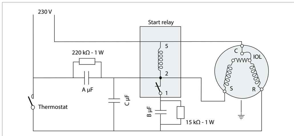
**Single phase - CSR wiring without trickle circuit**
